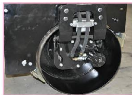
American brand hydraulic motor drive the front drum walking
