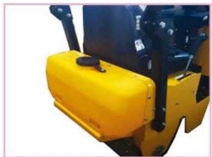
Plastic water tank free from corrosion and convenient for the water-spraying
