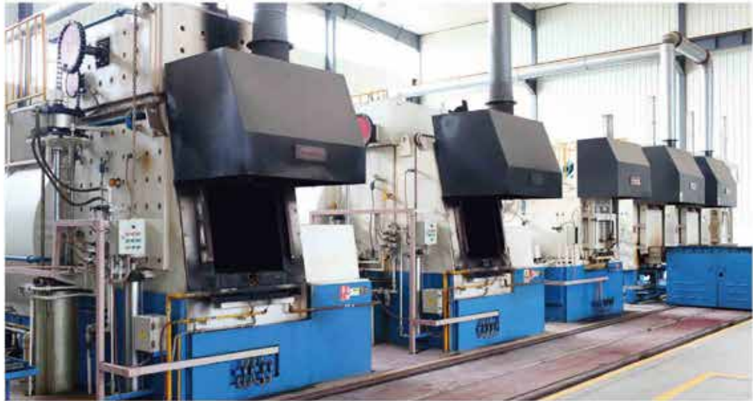
热处理流水线 (包括气体渗碳氮化炉) Heat Treatment Production Line(Gas Carburizing Nitriding Furnace included)
