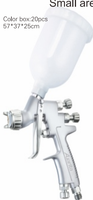
Mini H-921 Standard nozzle: 0.8/1.0/1.2mm Optimal pressure: 2.0bar/29psi Maximum pressure: 2.5bar/36psi Air consumption: 5~7cfm Pattern width: about 150mm Spray distance: 150mm Cup capacity: 250 ml
