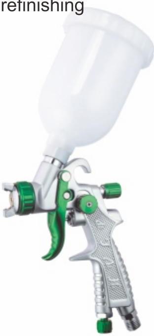
H-891 Standard nozzle: 0.8/1.0/1.2mm Optimal pressure: 2.0bar/29psi Maximum pressure: 2.5bar/36psi Air consumption: 5~7cfm Pattern width: about 130mm Spray distance: 150mm Cup capacity: 250 ml
