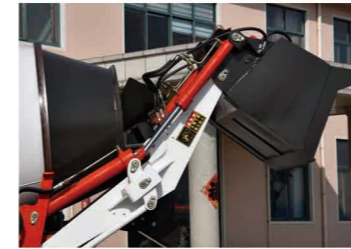
铲斗下翻功能 ，实现装载功能，真正实现一机多用功能 The bucket is turned down to achieve the loading function. Realize a multi-purpose function
