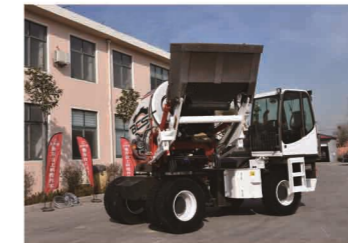
车型可选：驾驶室左前方与动臂滚筒同时左右旋转，驾驶室左后方可前后双向驾驶 The vehicle can be selected: the cab is in the front-left : the moving arm drum and the cab can be rotated at the same time the cab is in the left rear : the mixer can drive bi-directionally.
