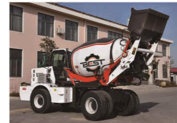
车型可选：驾驶室左前方与动臂滚筒同时左右旋转，驾驶室左后方可前后双向驾驶 The vehicle can be selected: the cab is in the front-left : the moving arm drum and the cab can be rotated at the same time the cab is in the left rear : the mixer can drive bi-directionally.
