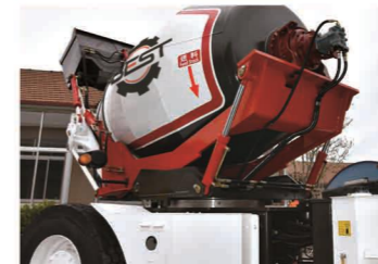
可前倾式卸料功能使卸料更彻底，速度更快 The dumping function can make the unloading more thorough and faster.
