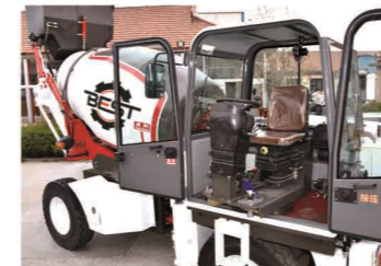
驾驶室操作台可旋转，前后双向驾驶更方便 The cab operating table can be rotated, and the mixer can drive bi-directionally. It is more convenient.
