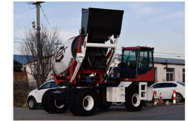
车型可选： 驾驶室左前方 与动臂滚筒同时左右旋转， 驾驶室左后方 可前后双向驾驶 The vehicle can be selected: the cab is in the front-left: the moving arm drum and the cab can be rotated at the same time the cab is in the left rear: the mixer can drive bi-directionally.
