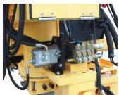
12. With Italy quick plugs to connect hydraulic power, smooth insertion and extraction, no oil leak
