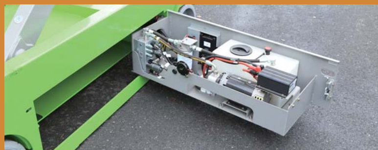
Swing-out trays on two sides
