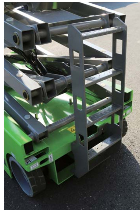
Antiskid ladder with 10mm thickness
